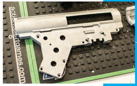
A prototype Evo gearbox casing, notably lacking the ovalised cylinder window.
