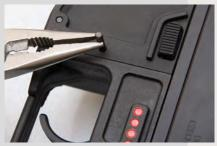
Push out the smaller retainer pin, this might require a pin-punch or pliers.
