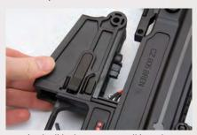
Simply slide the new mag well into place and replace both pins.
